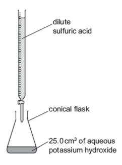
A student titrated 25.0 cm3 of 0.0500 mol/dm3 aqueous potassium hydroxide with dilute sulfuric acid in the presence of an indicator. The volume of dilute sulfuric acid needed to neutralise the aqueous potassium hydroxide was 20.0 cm<sup>3</sup>.
