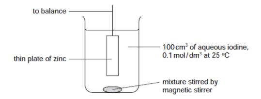
The mass of the zinc plate was measured every minute until the reaction was complete.
