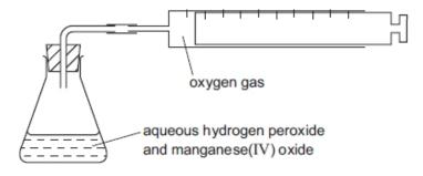
40 cm<sup>3</sup> of aqueous hydrogen peroxide was put in the flask and 0.1 g of small lumps of manganese(IV) oxide was added. The volume of oxygen collected was measured every 30 seconds. The results were plotted to give the graph shown below.
