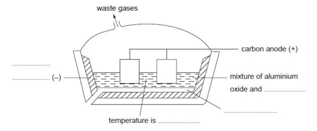
(c) The ions that are involved in the electrolysis are Al3+ and O2-. (i) Write an equation for the reaction at the cathode.
