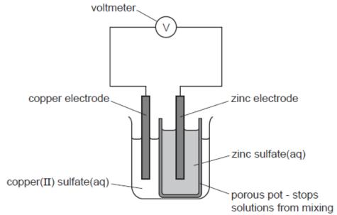
(i) Give an explanation for the following in terms of atoms and ions. observation at zinc electrode - the electrode becomes smaller explanation observation at copper electrode - the electrode becomes bigger explanation ...... \_\_\_\_\_[1] (ii) When a current flows, charged particles move around the circuit. What type of particle moves through the electrolytes? [1] Which particle moves through the wires and the voltmeter? [1]
