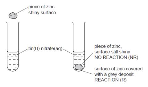
This experiment could be carried out with other metals and the results recorded in a table. Then the order of reactivity can be deduced.
