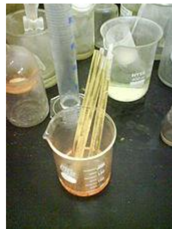
Freshly prepared aqua regia is colorless, but it turns orange within seconds. Here, fresh aqua regia has been added to these NMR tubes to remove all traces of organic material.
