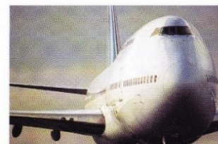
Aircraft bodies are made from alloys of aluminium because these alloys are strong yet lightweight.
